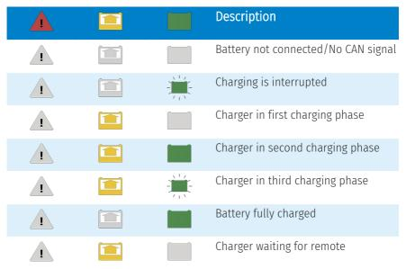
Tab. 1: Display of the operating status LEDs
